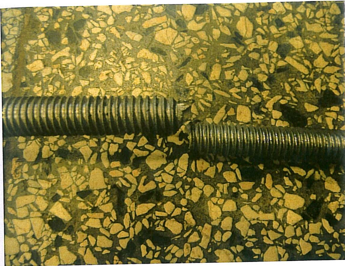
Fig. 5: Failure in the threads of the roping device
