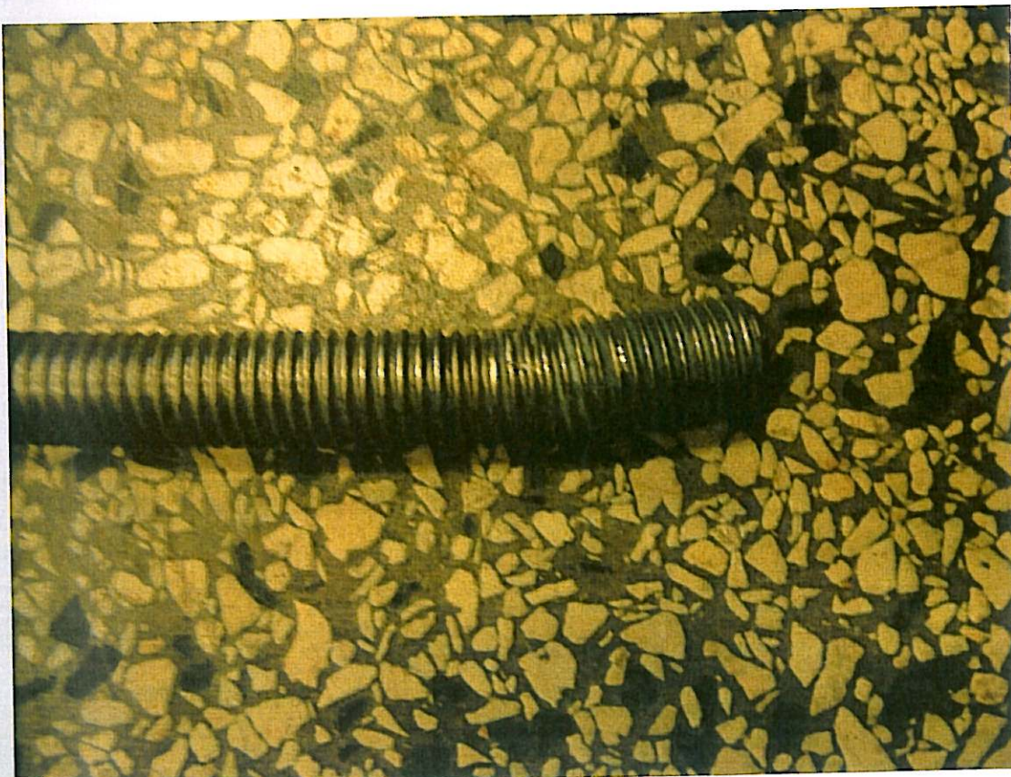
Fig. 6: Local bending of the threads due to deformation of the hollow section
